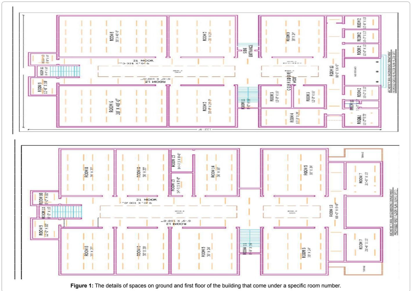
Figure 1: The details of spaces on ground and first floor of the building that come under a specific room number.
