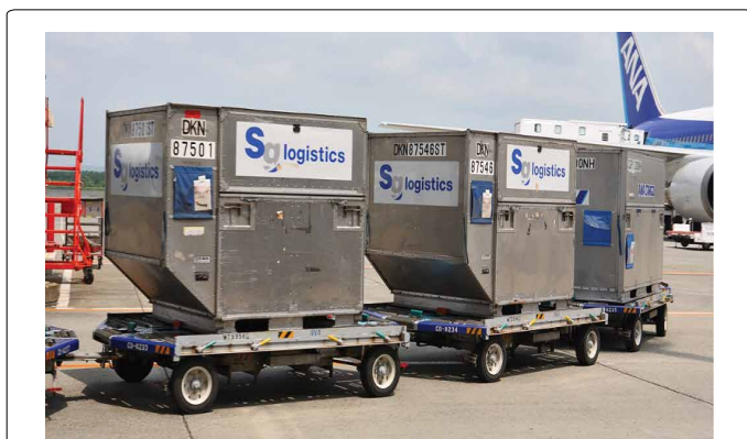
Figure 5: Figure showing light aluminium air-freight container.
