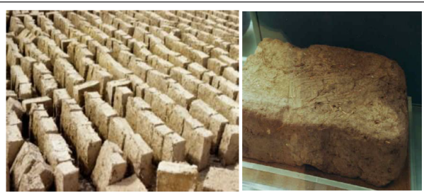
Figure 1: Composite bricks made out of straw and mud.
