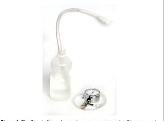
Figure 1: The Blow bottle system and a pressure manometer. The pressure is adjusted by varying the quantity of water in the bottle.
