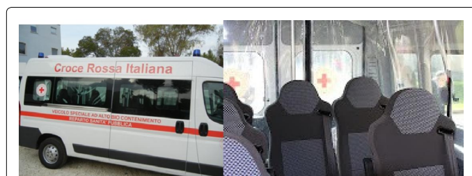
Figure 4: Fiat Ducato Combi Flex Floor 2.3 to 9 people arranged with insulation module BETH-RL and with a unit-filter pressurized at high efficiency HEPA (High Efficiency Pa reticular Air).
