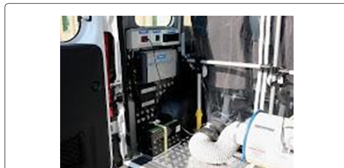
Figure 5: A filter unit external pressurization HEPA ensures the control of the air flow, variable and adjustable according to the number persons transported and the negative internal pressure (Pascal 80/10/50).
