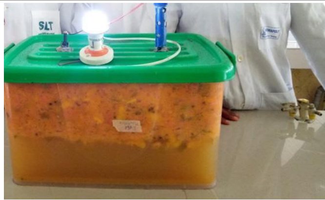
Figure 2: The bioelectricity lights up a 2V bulb.
