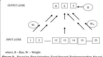
**Figure 2:** Bayesian Regularization Feed-forward Backpropagation Neural Network showing the connections between the computing units
