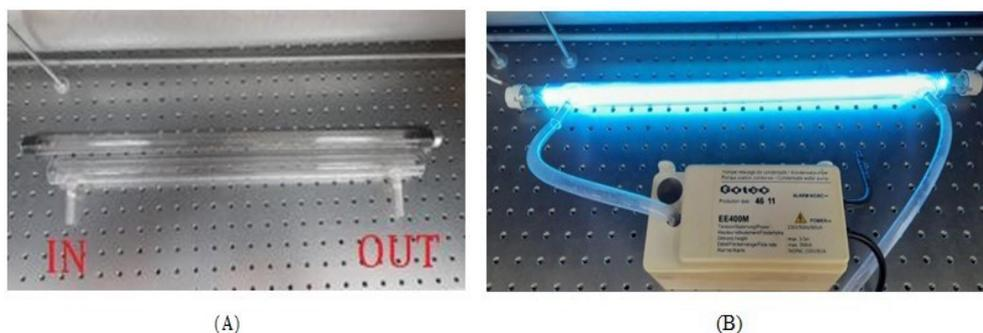
**Figure 2:** (A) The decontamination device consists of the lamp (UV) and the quartz tube with 2 holes that serve as input- output (IN-OUT) decontamination solution and (B) the decontamination device connected to a pump source.
