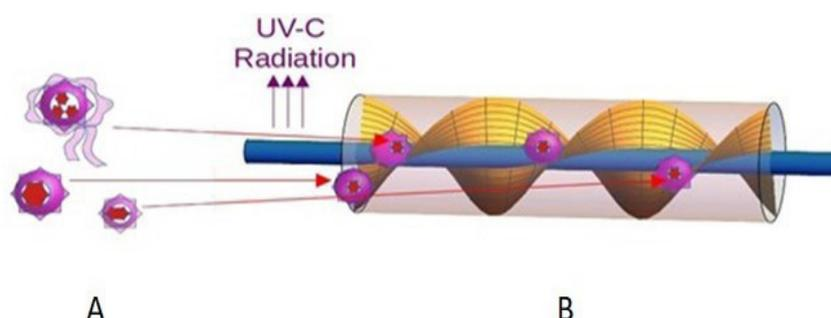
**Figure 1:** The pathogen droplets. (A) with dimensions about 10-100 nm can be pumped and imposed under rotation acceleration between free space of helical ensemble of the scrolled fibers and (B) Achieving the evanescent zone of UVC radiation of each fiber the pathogens can be effectively inactivated.
