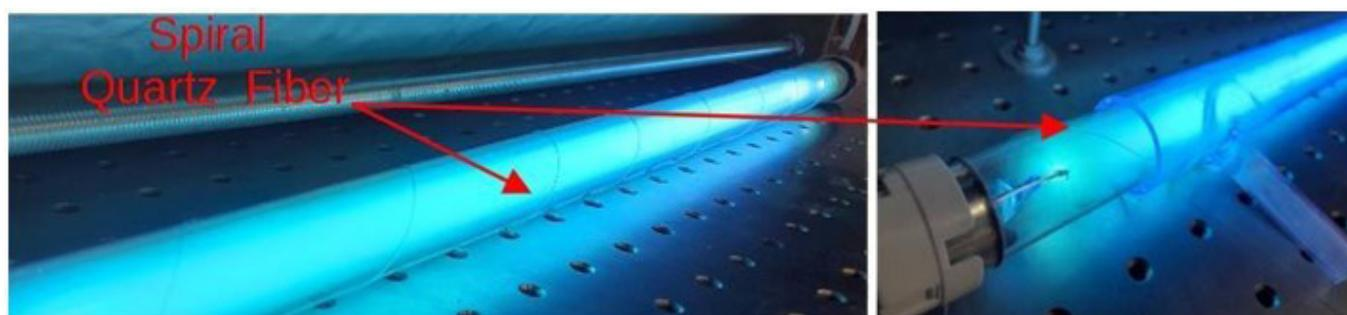
**Figure 3:** Here is shown the quartz fiber spiral located between the UV lamp and the tube which serves for the rotation effect of molecules, bacteria and pathogens when the contaminated liquid flows through the tube.
