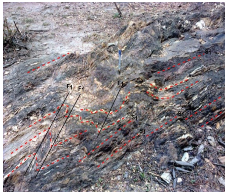
Plate I: Quartzite veinlet invading schist showing F1 folding and S1 Schistosity
