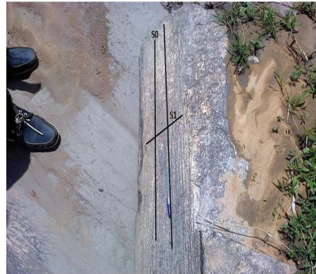
Plate II: S1 Schistosity on S0 surface on muscovite schist
