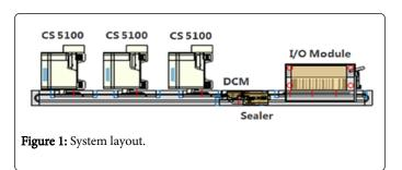
**Analytical modules:** Three Sysmex CS-5100 automated coagulation analyzers.
