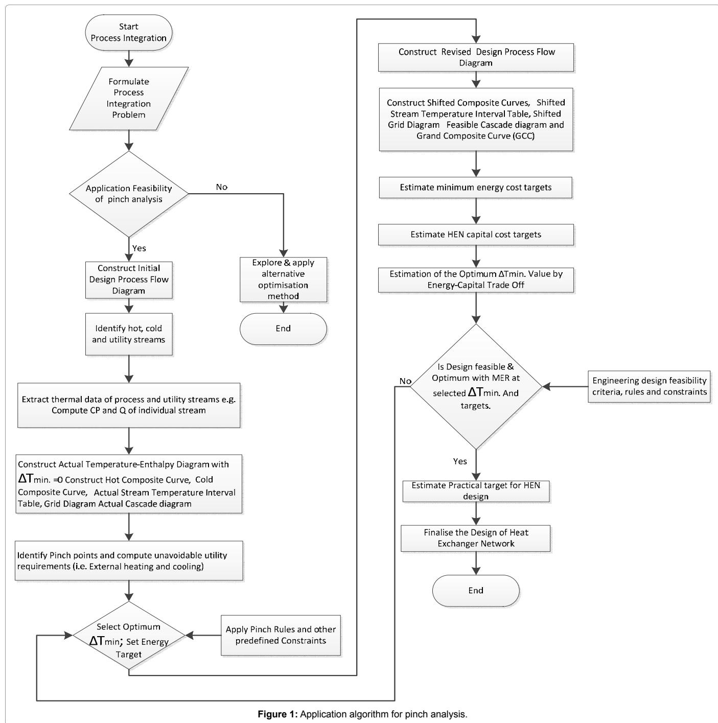
Figure 1: Application algorithm for pinch analysis.
