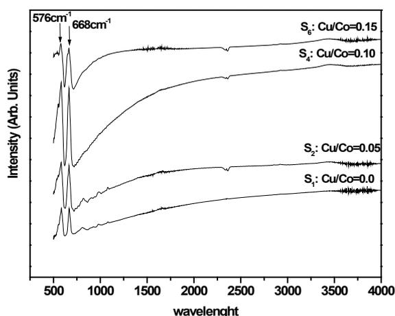
Figure 4: FT-IR Intensity Results for Cu-Co Oxides Nano-Crystals with Different Cu/Co Mole Ratios.
