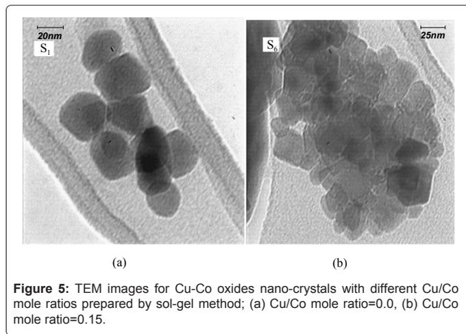
Figure 5: TEM images for Cu-Co oxides nano-crystals with different Cu/Co mole ratios prepared by sol-gel method; (a) Cu/Co mole ratio=0.0, (b) Cu/Co mole ratio=0.15.
