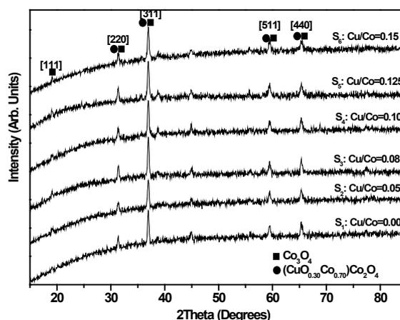
Figure 3: XRD patterns of Cu-Co oxides nano-particles with different Cu/Co mole ratio.
