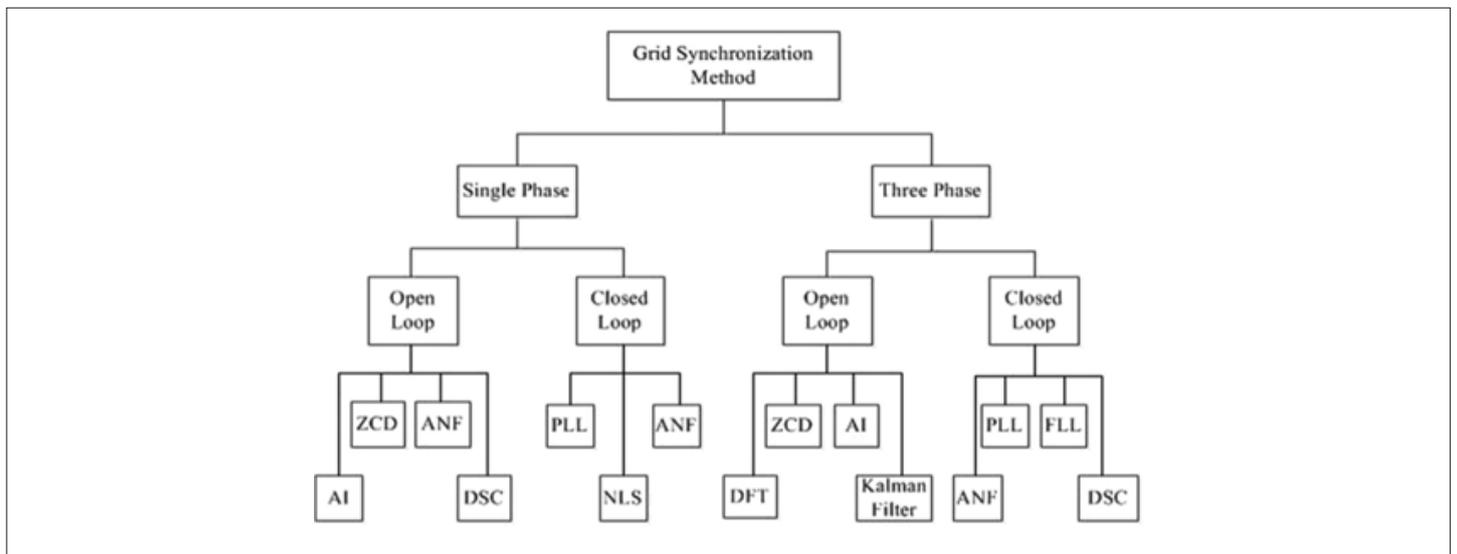
Figure 4: Various grid synchronization methods under respective categories.
