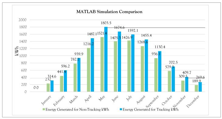
Figure 9: MATLAB simulation model comparison between tracking and non-tracking output.
