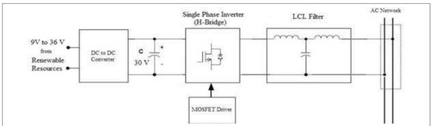
Figure 3: Basic diagram to connect solar panel system to the main grid.
