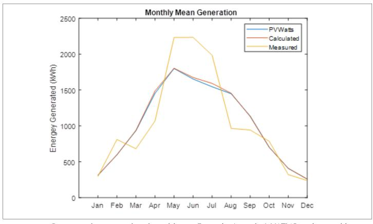
Figure 7: Comparison of mean output for each month between Fronius data (orange line), MATLAB simulation model (red line) and PVWatts simulation model (blue line).
