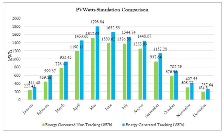
Figure 8: PVWatts simulation model comparison between tracking and non-tracking output.
