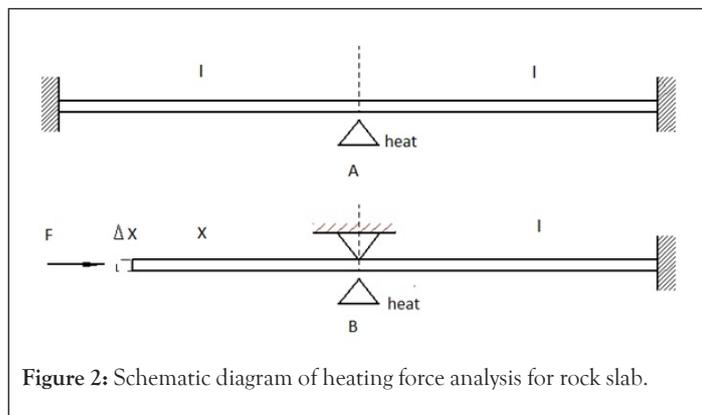
Figure 2: Schematic diagram of heating force analysis for rock slab.
