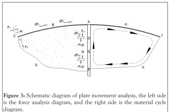
Figure 3: Schematic diagram of plate movement analysis, the left side is the force analysis diagram, and the right side is the material cycle diagram.
