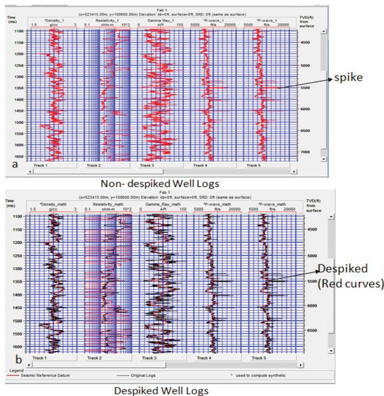
Figure 2: Well log correction showing (a) original well logs with spike and (b) despiked well logs (red curve).
