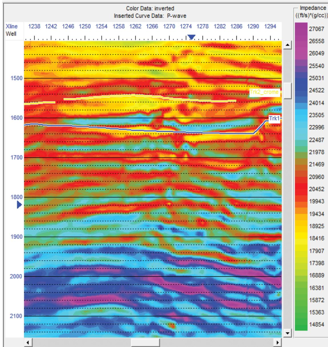
Figure 9: The inverted acoustic impedance volume showing overpressure variations in the field.
