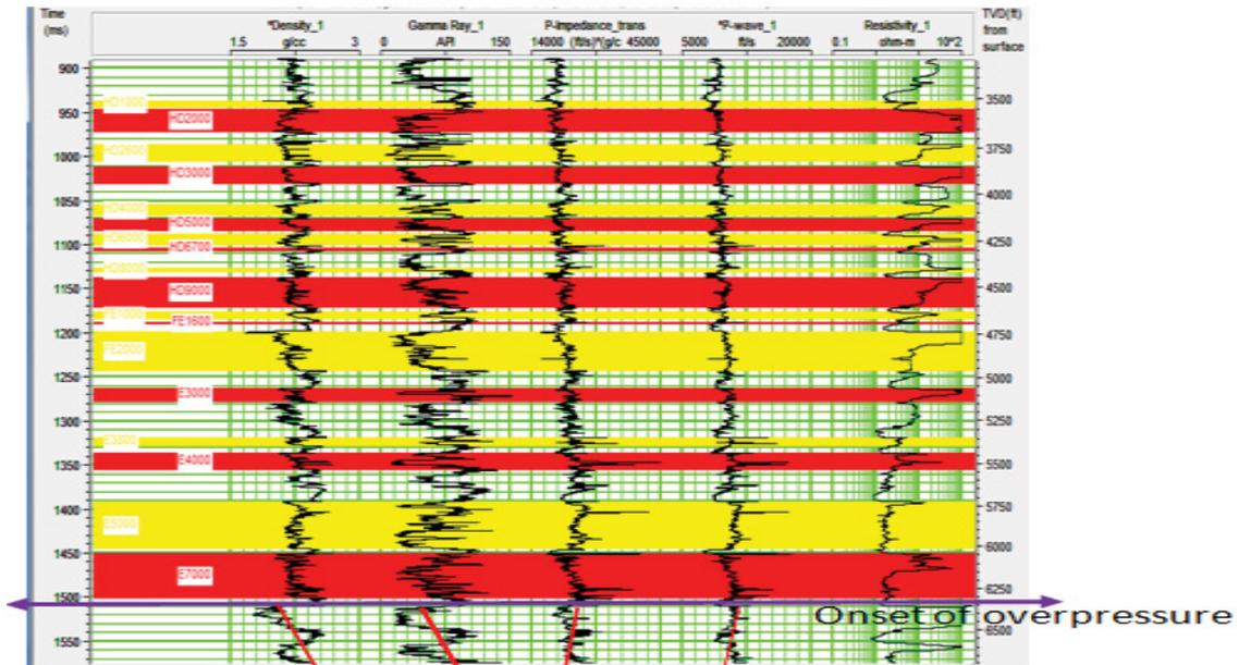
Figure 6: Density, gamma ray, acoustic impedance, P-wave and resistivity logs, showing reservoir horizons and trend line behavioral pattern and deviation indicating overpressure zones.
