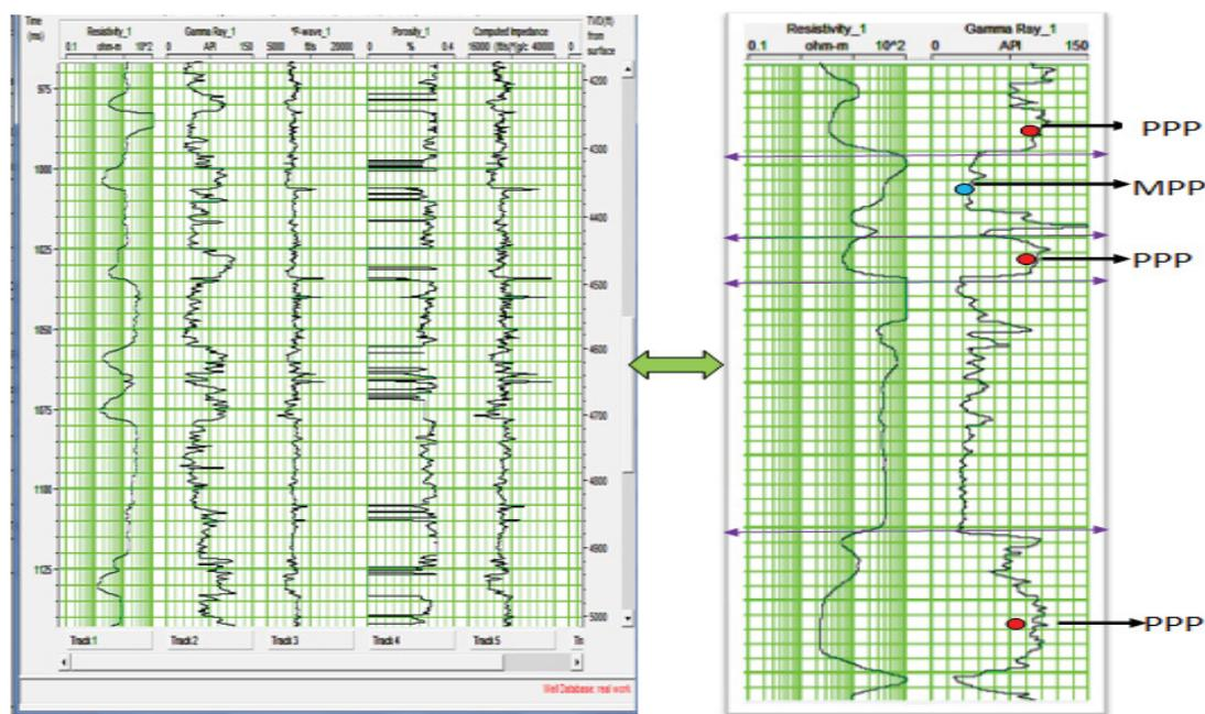
Figure 4: Predicted pore pressure (PPP) points picked from shale depth intervals (red dots) and measured pore pressure (MPP) points in the sands (blue dots).
