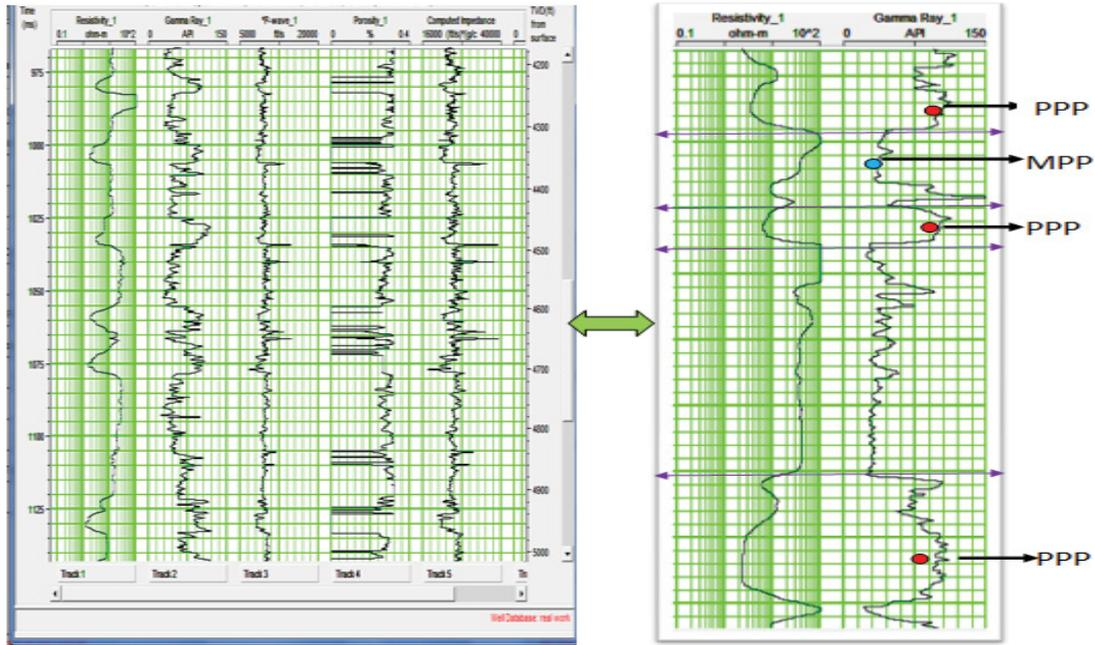
Figure 6: Total vertical stress and normal compaction trend line (blue line) generated from density, P-wave, gamma ray, resistivity, acoustic impedance logs showing onset of overpressure at the normal compaction points of deviations (red line).
