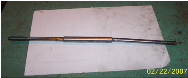
Figure 6: Shaft showing the line of bending.
