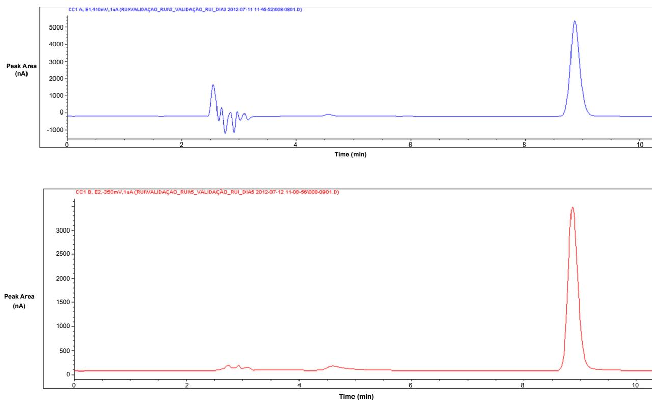
Figure 2: Chromatogram of MN at 15 nmol\*mL<sup>-1</sup>; (a) E1-Oxidation, (b) E2-Reduction (down); retention time (MN) of 8.873 min.
