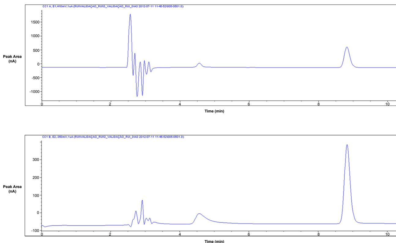
Figure 1: Chromatogram of MN at 2 nmol·mL<sup>-1</sup>; (a) E1-Oxidation, (b) E2-Reduction (down); retention time (MN) of 8.873 min.
