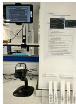
(b) Store installation. The Bluetooth barcode scanner works in manual mode
