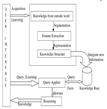
Fig. 2.1 Knowledge Base System Model/Architecture
