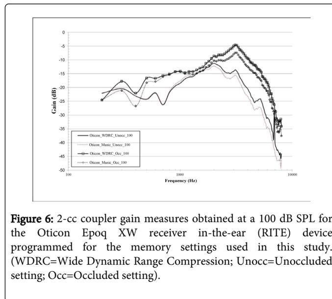
**Figure 6:** 2-cc coupler gain measures obtained at a 100 dB SPL for the Oticon Epoq XW receiver in-the-ear (RITE) device programmed for the memory settings used in this study. (WDRC=Wide Dynamic Range Compression; Unocc=Unoccluded setting; Occ=Occluded setting).
