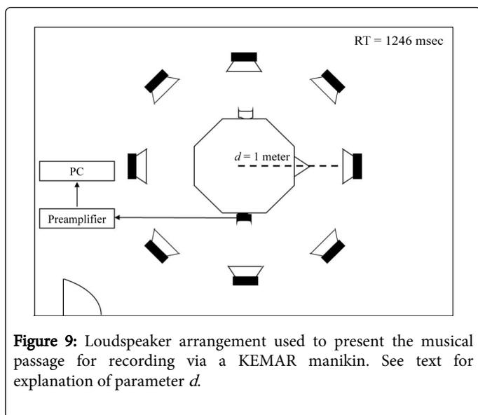
**Figure 9:** Loudspeaker arrangement used to present the musical passage for recording via a KEMAR manikin. See text for explanation of parameter *d*.
