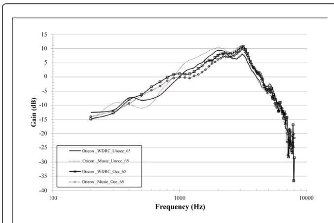
**Figure 3:** 2-cc coupler gain measures obtained at a 65 dB SPL for the Oticon Epoq XW RITE device programmed for the memory settings used in this study. (WDRC=Wide Dynamic Range Compression; Unocc=Unoccluded setting; Occ=Occluded setting).
