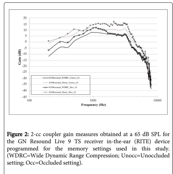
**Figure 2:** 2-cc coupler gain measures obtained at a 65 dB SPL for the GN Resound Live 9 TS receiver in-the-ear (RITE) device programmed for the memory settings used in this study. (WDRC=Wide Dynamic Range Compression; Unoc=Unoccluded setting; Occ=Occluded setting).
