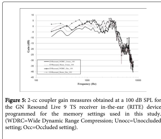
**Figure 5:** 2-cc coupler gain measures obtained at a 100 dB SPL for the GN Resound Live 9 TS receiver in-the-ear (RITE) device programmed for the memory settings used in this study. (WDRC=Wide Dynamic Range Compression; Unocc=Unoccluded setting; Occ=Occluded setting).
