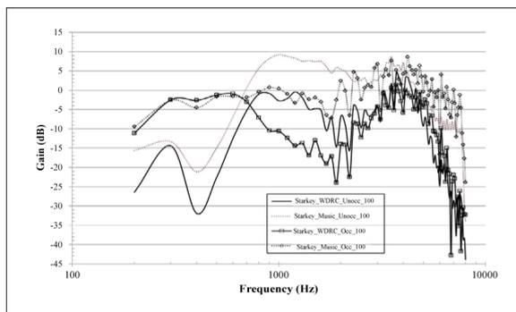
**Figure 7:** 2-cc coupler gain measures obtained at a 100 dB SPL for the Starkey Wi Series i110 receiver in-the-canal (RIC) 312 device programmed for the memory settings used in this study. (WDRC=Wide Dynamic Range Compression; Unocc=Unoccluded setting; Occ=Occluded setting).
