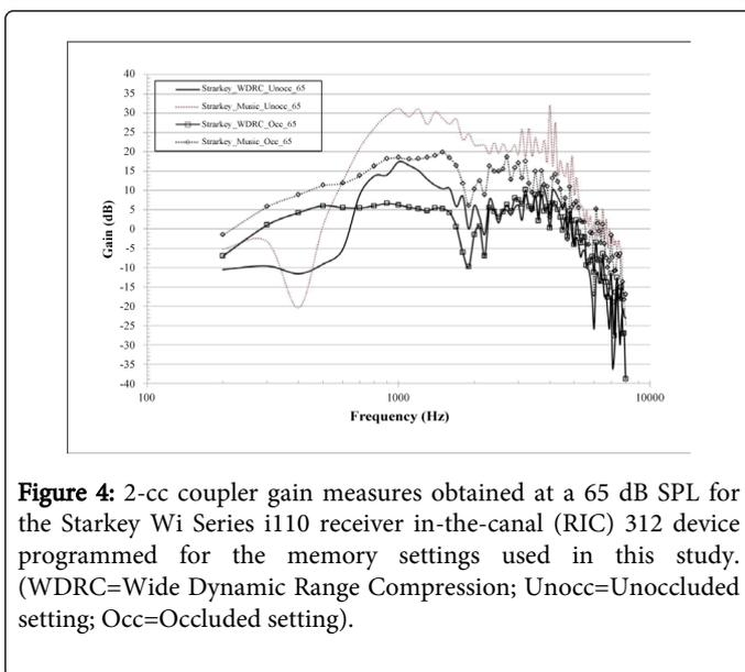
**Figure 4:** 2-cc coupler gain measures obtained at a 65 dB SPL for the Starkey Wi Series i110 receiver in-the-canal (RIC) 312 device programmed for the memory settings used in this study. (WDRC=Wide Dynamic Range Compression; Unocc=Unoccluded setting; Occ=Occluded setting).
