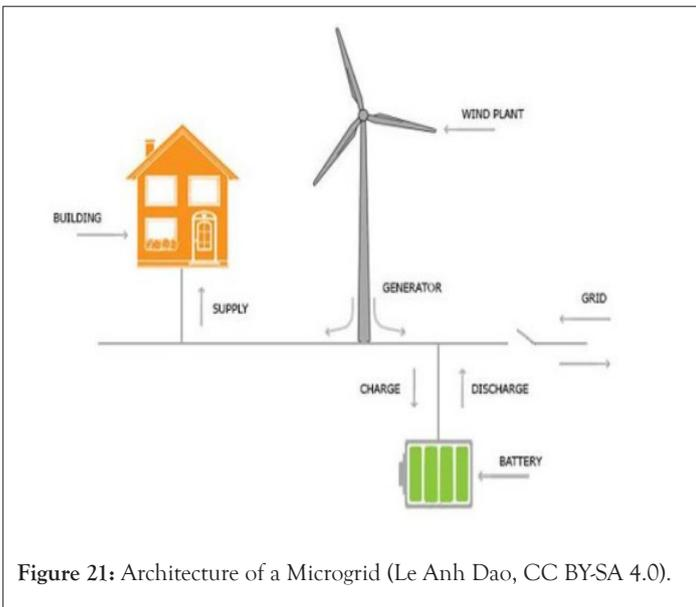
Figure 21: Architecture of a Microgrid (Le Anh Dao, CC BY-SA 4.0).
