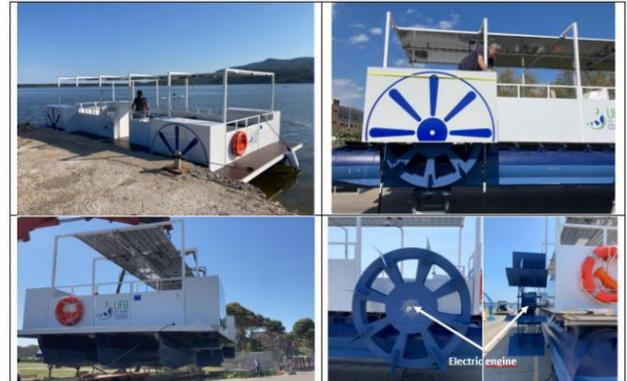
Figure 18: The 'Valentino III'- Different views of the Valentino II e-boat, i.e. the innovative LIFE e-boat equipped with four independent paddle wheels connected to as many independent engines, prepared for autonomous driving.
