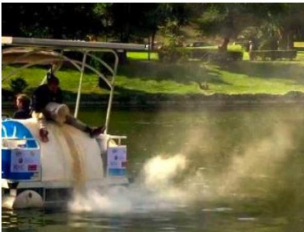
Figure 17: Bioremediation in EUR pond: A picture taken in Rome (2016) during the bioremediation in EUR pond made through an e-boat prototype. A particular species of bacteria were introduced into the pond for sanitization.
