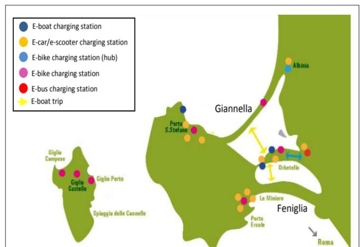
**Figure 2:** Map of the mobility system; in purple, the e-boat charging stations; in orange, the e-car/e-scooter charging stations; in blue, the e-bike hub charging stations; in pink, e-bike charging stations; in red, e-bus charging stations and in yellow, the e-boat trips. **Note:** (●) E-boat charging station; (●) E-car/e-scooter charging station; (●) E-bike charging station (hub); (●) E-bike charging station; (●) E-bus charging station; (●) E-boat trip.
