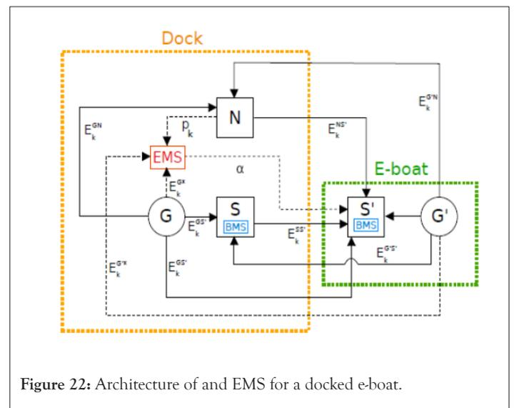
Figure 22: Architecture of and EMS for a docked e-boat.
