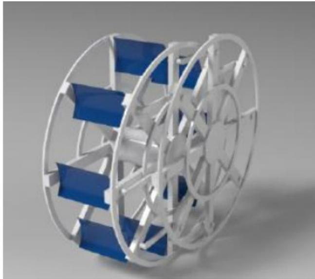
Figure 16: E-boat paddle wheel designed by POMOS.
