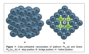
In the present work we studied processes of platinum stable nanoclusters and binary nanoclusters  $Pt_nX_m$  (X - Fe, Co, Ni; n=42; m=13) interaction with carbon monoxide. The nanoclusters were of the core-shell structure.
