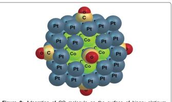
Figure 2: Adsorption of CO molecule on the surface of binary platinum nanocluster  $Pt_{42}Co_{13}$ .
