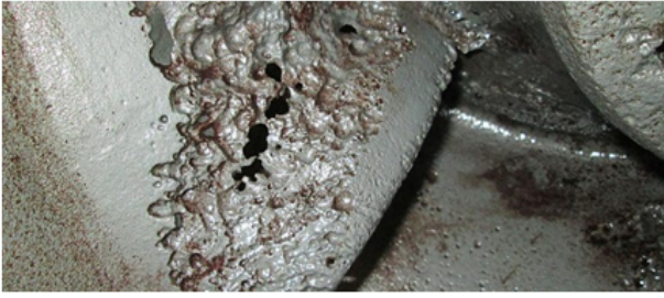
Figure 1: Defected impeller by cavitation
