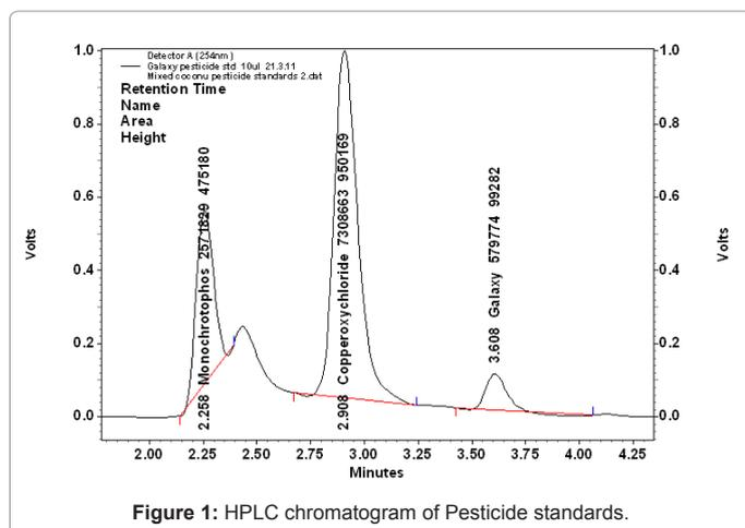
Figure 1: HPLC chromatogram of Pesticide standards.
