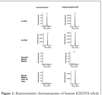
**Figure 2**: Representative chromatograms of human K2EDTA whole blood spiked with Acetaminophen-D4. The figure was created using Graph Pad 8 based on the output from Sciex Analyst version 1.6.2.
