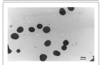
**Figure 5:** TEM of high molecular weight star polymethylmethacrylates.
