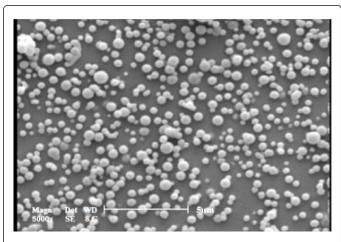
**Figure 4:** SEM of high molecular weight star polymethylmethacrylates.
