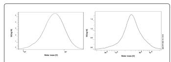
**Figure 2:** GPC graph of hydrolyzed star polymers, (a) PMMA  $([M]_o:[I]_o \text{ of } 800:1)$ ; (b) PMMA  $([M]_o:[I]_o \text{ of } 16000:1)$ .
