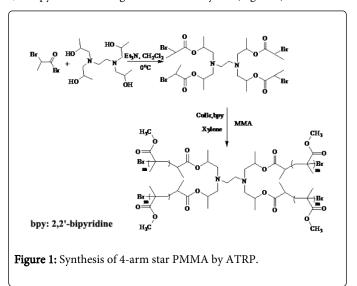
The reaction must be operated in inert atmosphere to avoid termination of living polymerization due to CuBr oxidation.
