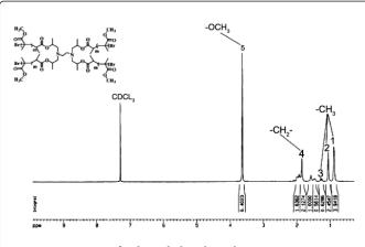
Figure 3: 1H-NMR of polymethylmethacrylates.
