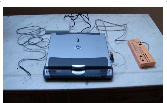
Figure 1B: Photography of the device. 1. Rectal catheter; 2. Analyser of sensors data; 3. Computer; 4. Insulin pump.
