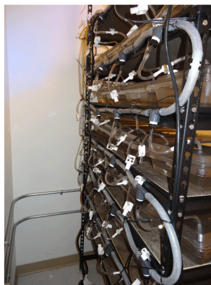
Figure 3: Back view of assembled water system. This shows the "S" form that allows water to go from the UV sterilizer to the individual tanks (photo).
