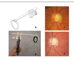
**Figure 1:** Smartphone retinal imaging system. (A) Computer Aided Design (CAD) of the retinal imaging adapter. (B) A functional prototype of the device on an iPhone 6 plus. (C) Smartphone captured image of a glaucomatous disc. (D) Image of the glaucomatous disc taken with a conventional fundus camera.
