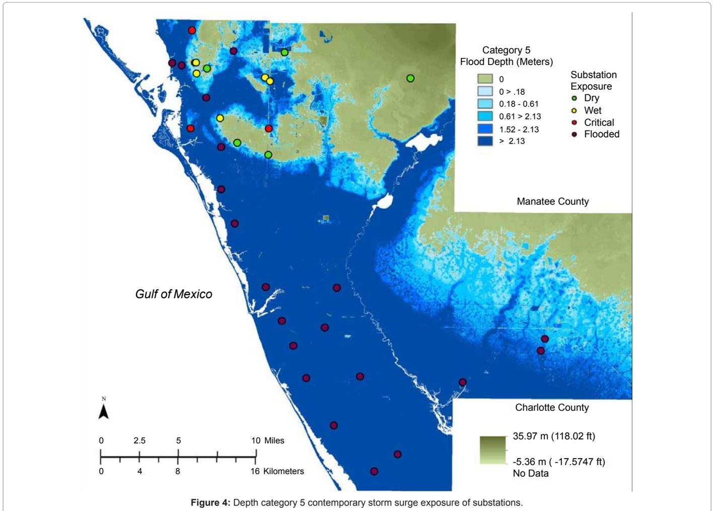
**Figure 4:** Depth category 5 contemporary storm surge exposure of substations.
