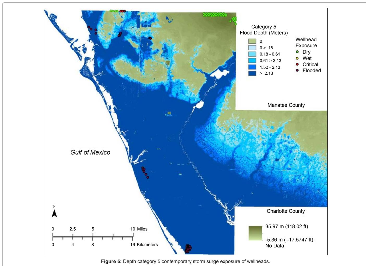
Figure 5: Depth category 5 contemporary storm surge exposure of wellheads.
