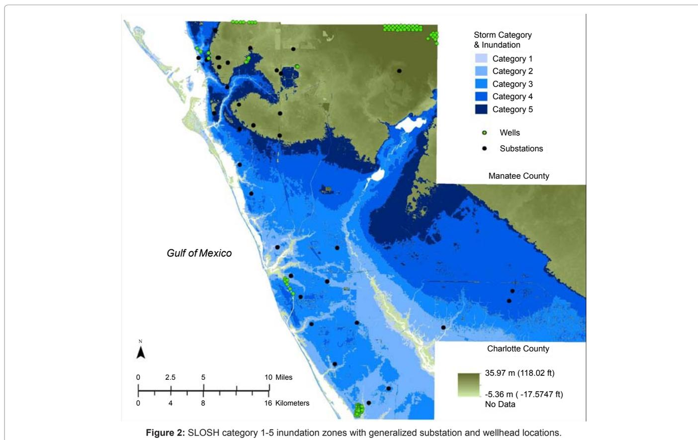
Figure 2: SLOSH category 1-5 inundation zones with generalized substations and wellhead locations.
