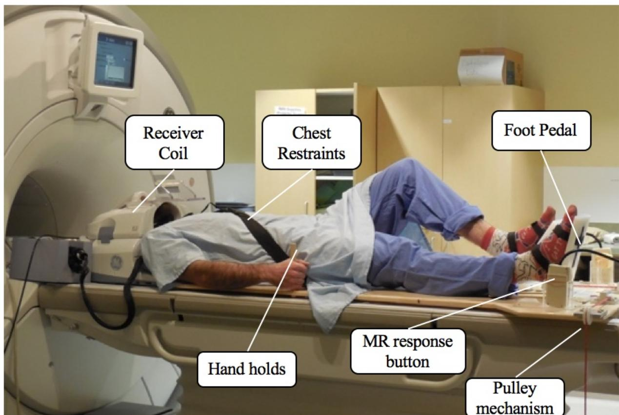
**Figure 2:** MR apparatus in the MR scanner with participant positioned for stepping movements. This device is modular within the scanner for individuals of varying height and weights.
