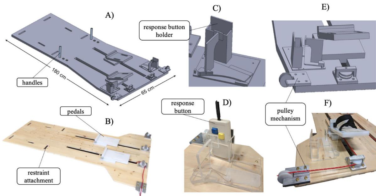
**Figure 1:** A CAD design of the MR apparatus including dimensions to assist with scale. This figure shows A) the dimensions and handholds, B) the pedals and their tracks, C) response button holders to time stamp stepping and hand holds for participants, D) the response button switch, E) pulley system in CAD and F) pulley system after fabrication.
