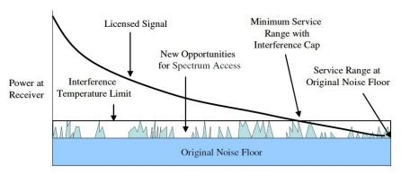
Fig 3: Interference Temperature Model [21]
