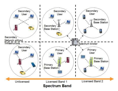
Fig 2: A Cognitive Radio Network Architecture with Primary and Secondary User Networks
