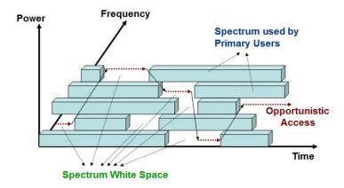
Fig 1: Spectrum Usage – Opportunistic Access of Spectrum White Space and Channel Switching by a Cognitive Radio User
