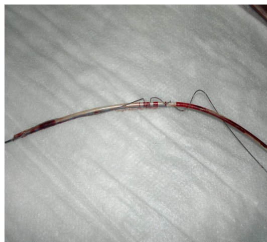
Figure 3: Image showing the ruptured shaft of the thrombus aspiration catheter. The catheter can be seen twisted on the guidewire leading to entrapment of the system in the RCA.
