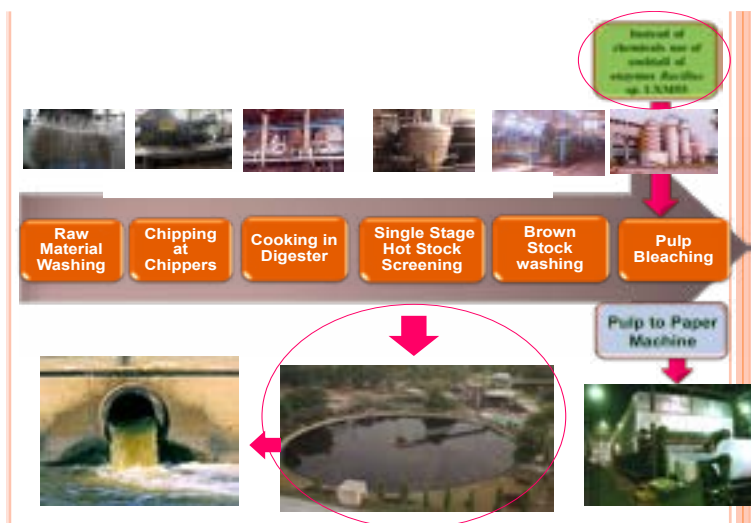
Figure: Pulp making process and use of cocktail enzyme from Bacillus sp. LXM 55 for pulp biobleaching
