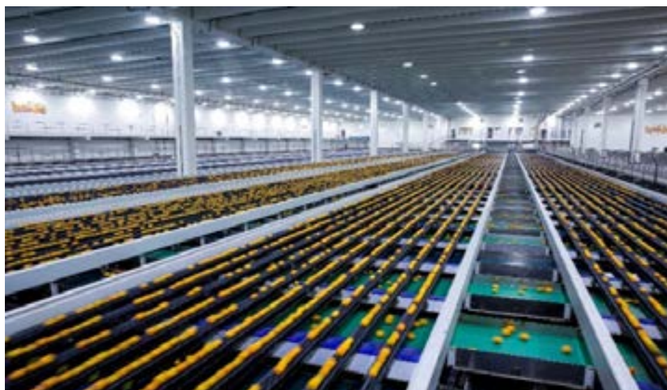
Figure 1: A typical layout of a lane sorting machine, showing the challenge of complexity and compliance.
