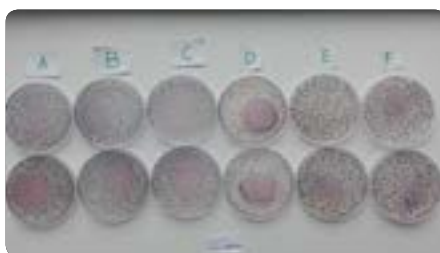
Figure 1: Coliform Count Plates: A-tap water (control), B-distilled water (control), C alkaline, D-acidic, E-silvered, F-8% concentration of hydrogen peroxide (currently approved disinfectant)
