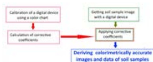
Figure1: Schematic diagram of obtaining a colorimetrically accurate image using digital devices
