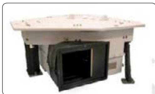
Figure 1: JIRAM optical head. It is mounted on the Juno spacecraft aft deck. All the white panels are radiators for both the detectors and the body of the instrument. JIRAM is passively cooled down to 80K
