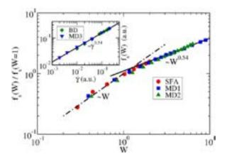
Rescaled shear stress as a function of Weissenberg number on double-logarithmic scales. The universal scaling plot allows for superposition of data from MD simulations, Brownian dynamics simulations and SFA experiments. Inset: Shear stress as function of shear rate.
