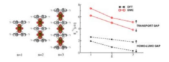
**Figure 1:** Model of vanadium benzene full-sandwich molecules featuring ferromagnetically coupled vanadium atoms. Right:  $\uparrow -/\downarrow$ -spin gaps for vanadium-benzene full sandwich structures in DFT and QMC treatments.
