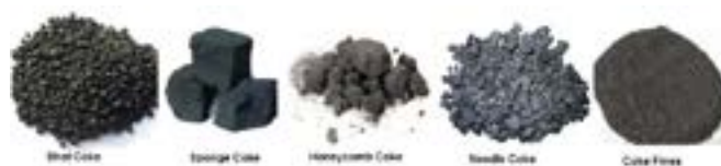
Figure.1: Different physical forms of high carbon content coke include shot coke, sponge coke, honeycomb coke, needle coke and coke fines. Coke can be 'green' or unprocessed, calcined, uncalcined, fuel grade, metallurgical grade or anode grade. Fouling Coke may be any one or a combination of these, with varying levels of purity.
