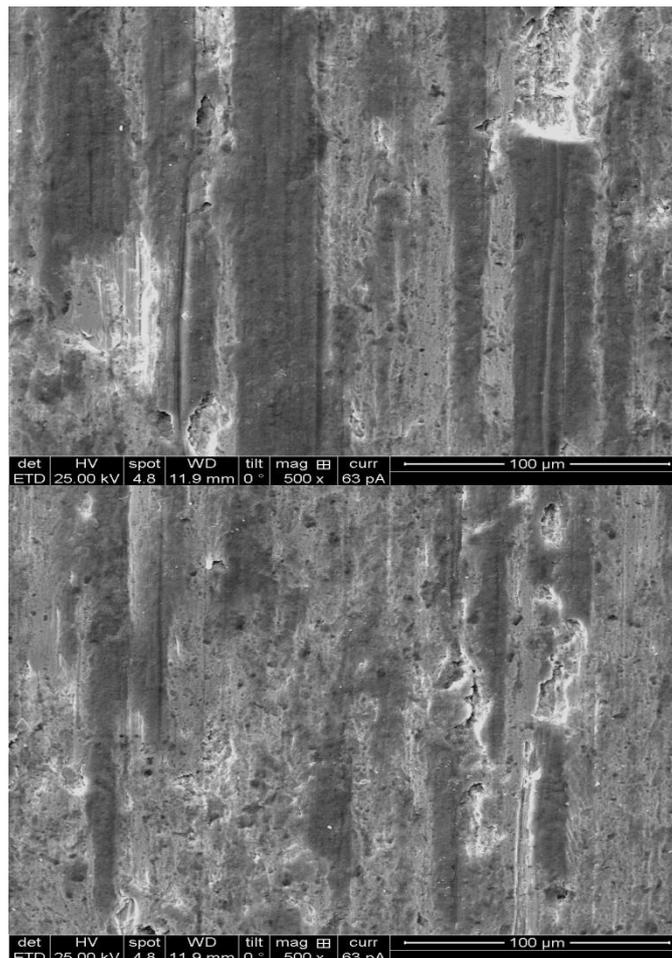
Fig. 4 Worn surface features of sample 1(a) 15 min (b) 30 min.
