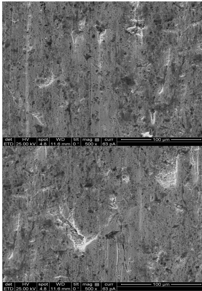
Fig. 5 Worn surface features of sample 3(a) 15 min (b) 30 min.
