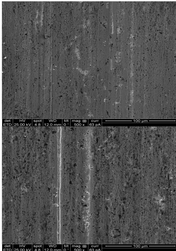
Fig. 6 Worn surface features of sample 5(a) 15 min (b) 30 min.
