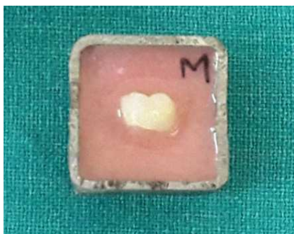
Fig 1: Crown fixed in metallic mould with buccal surface exposed
