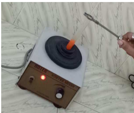
Fig 2: Agitating the undiluted test syrup in an agitator
