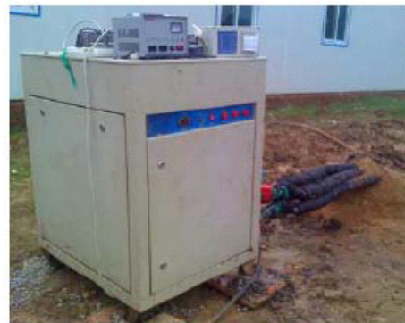
Figure 1: A part of view of field tests of the thermal performance of the BHEs Results and Discussion.
