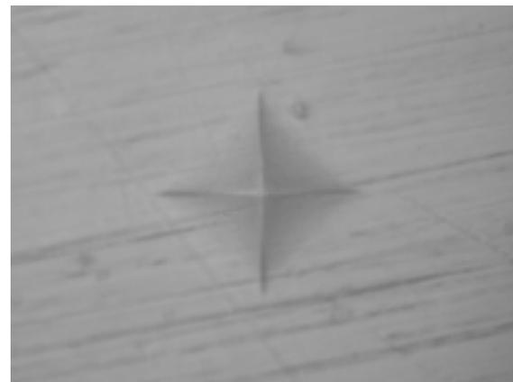
Figure 4: VH indentation of top surface FZ250 at room temperature.
