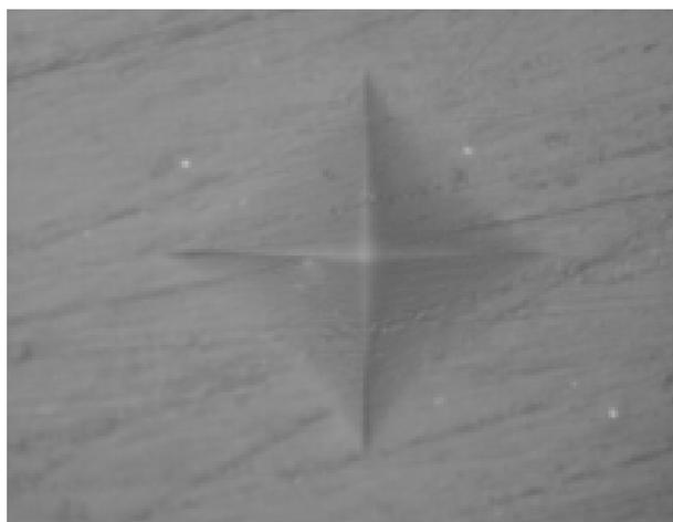
**Figure 7:** VH indentation of bottom surface TN at room temperature.
