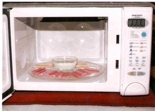
Fig. 4. Photograph showing specimens placed on the Turn table of oven along with the Borocil Bowl ( filled with water)
