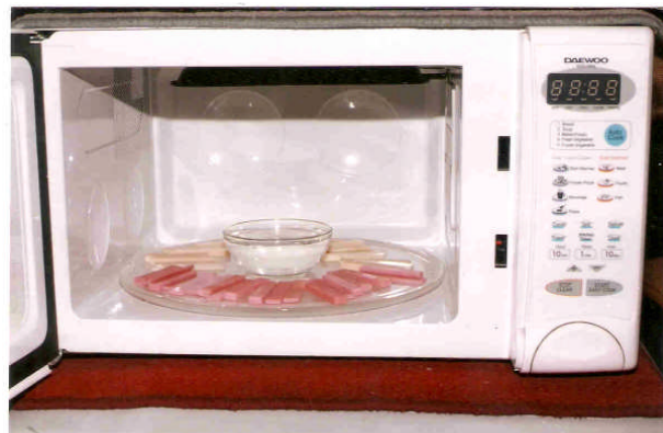
Fig. 3. Photograph showing specimens placed on the Turn table of oven along with the Borocil Bowl ( filled with water)
