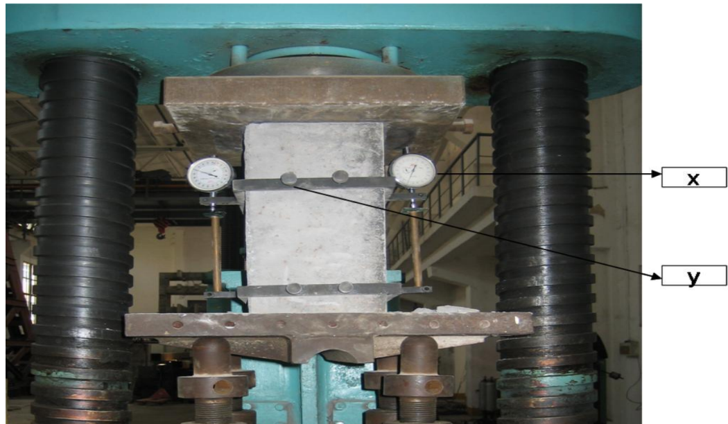
Figure 1. Test set up for static elastic modulus of elasticity (x = Compressometer, y = Testing ring)
