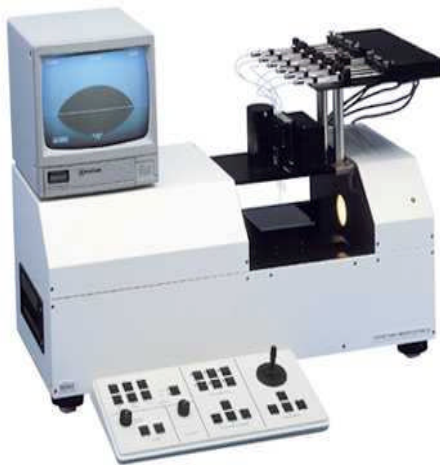
Fig.6. contact angle measured with optical microscope is shown on the computer screen attached to it
