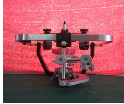
Fig.2. The wax rims are transferred to the Articulator with the aid of a facebow.
